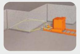
B picture showing Vertical Cutting of hard rock using Diamond rope.
