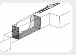
A Diagram showing horizontal cutting of hard rock using with Diamond rope.
